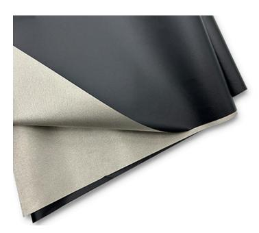
On the basis of ordinary conductive cloth increase nickel plating treatment. different from the general carbon black treatment, the surface composition is nickel metal, the black side also has good electrical conductivity, blackening after six times of treatment is more wearresistant not easy to fade, die cutting is not easy to burring, shielding effect is better.
